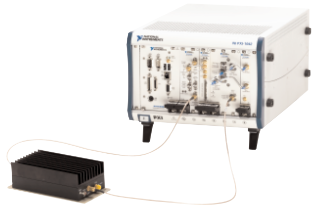
Figure 3. RF test system – PXI-5671 and PXI-5660
