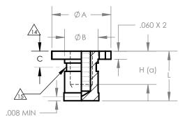
BLIND TAPPED STYLE FOR LONG LENGTHS ALL STEEL AND CRES SELF-LOCKING AND NONSELF-LOCKING ALUMINUM STYLE.
