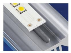
Liqui-Bond® EA 1805 is a two-component, epoxy based, liquid-dispensable adhesive. Liqui-Bond® EA 1805 has a thermal conductivity of 1.8 W/mK.
