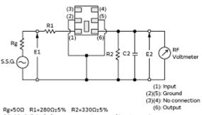
C2=10±2pF (Including stray capacitance and Input capacitance of RF voltmeter) E1: S.S.G. Output Voltage
