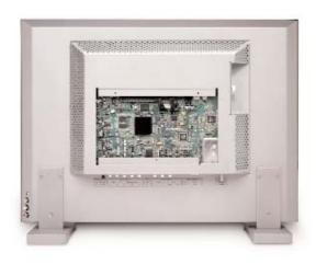
Zoran's SupraHD DTV Reference Design includes main board installed in flat panel display, stereo speakers, remote control, cables, preloaded software and documentation.
