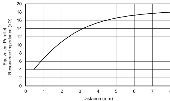
Figure 9. Typical R_p versus Distance With a 14-mm PCB Coil
