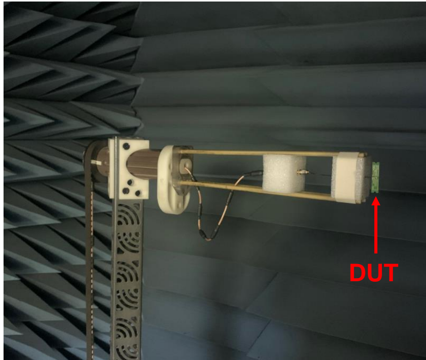
FIGURE4.1.2 ANTENNA IN FREE SPACE WITH OTA CHAMBER
