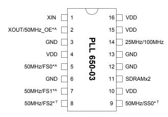
**Note:** SDRAMx2: Double Drive strength. <sup>T</sup>: Tri-Level input ^: Internal pull-up resistor \*: Bi-directional pin (input value is latched upon power-up).
