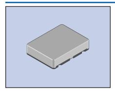
The VC-TXO-39SMX is a VC (Voltage Controlled)  $\ensuremath{\textbf{FEATURES}}$ TCXO (Temperature Compensated Crystal Oscillator) featuring very tight stability over a wide temperature range. The small SMD ceramic package measures 11.4 x 9.6 x 2.3 mm. The voltage control has a tuning range of  $\pm$  12 ppm typical. The low profile package is ideal for wireless communications applications.
