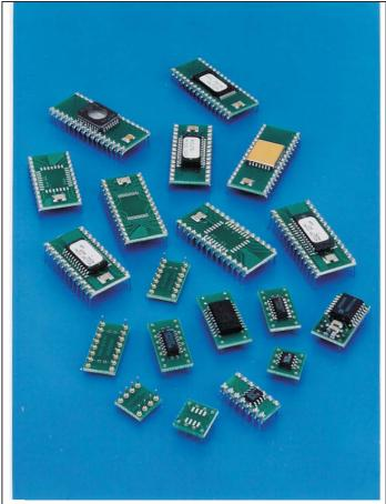
This new family of Accutek DIP Adapter Modules converts surface mount IC's to pin compatible DIP packages for creating drop-in replacements for end-of-life DIP IC's. Package types supported are: SOJ, PLCC, SOIC, SOP, TSOP, QSOP, HSOP, MSOP, LLP (Leadless Leadframe Package), CSP (Chip Scale Package) and CLCC.
