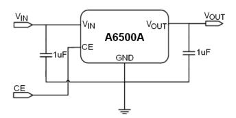
NOTE: Input capacitor (C<sub>IN</sub> = 1uF) and Output capacitor  $(C_{OUT} \ge 1uF)$  are recommended in all application circuit.
