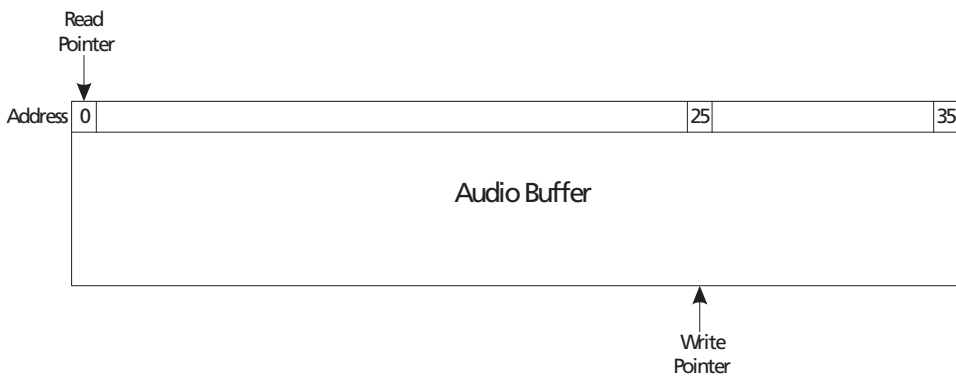
Figure 4-44: Audio Buffer After Initial 26 Sample Write
