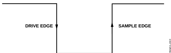
Figure 34. SPI Mode 3 SCLK Edges
