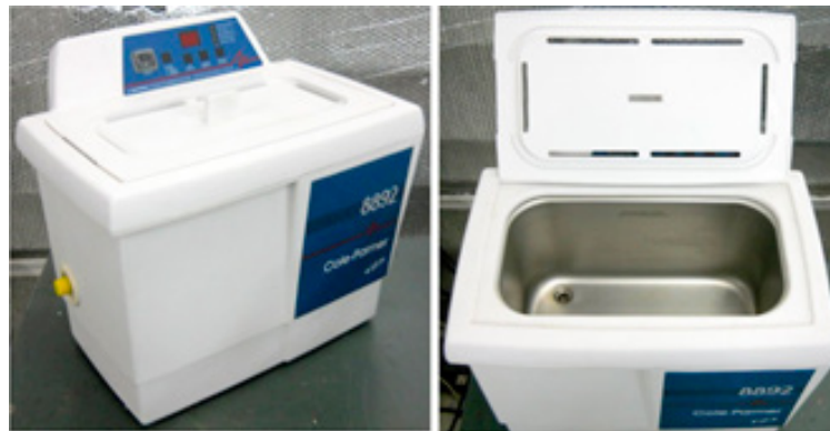
Figure 41. A small scale ultrasonic bath to remove flux residue. Shown here is Model 8892 ultrasonic cleaning tank from Cole-Palmer
