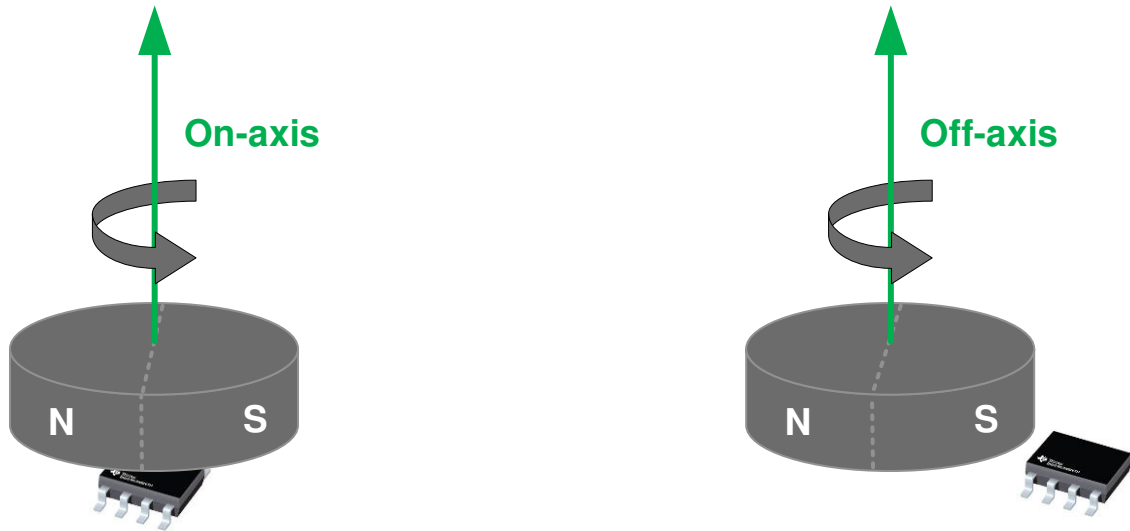
Figure 8-5. On-Axis vs. Off-Axis Angle Measurements
