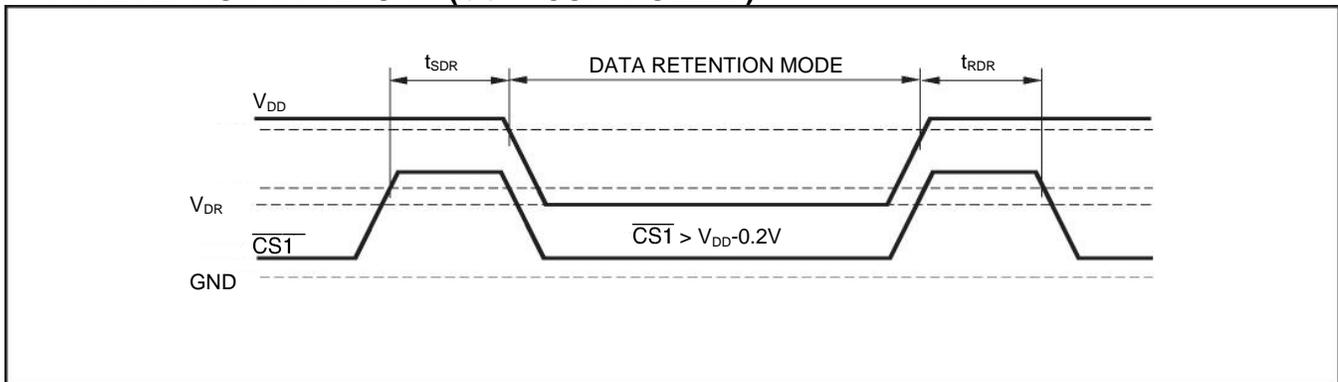
**DATA RETENTION WAVEFORM (CS2 CONTROLLED)**
