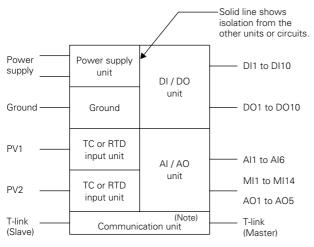
(Note) The communication unit is not isolated from the AI/AO unit when using T-link.
