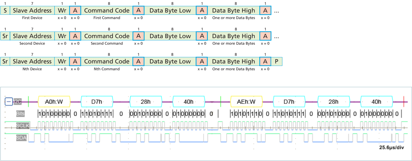
Figure 7 — DISABLE_FAULT COMMAND (D7h)_WRITE
