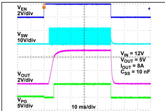
FIGURE 2-44: Enable Turn-On/Turn-Off.
