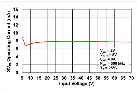
**FIGURE 2-28:**  $SV_{IN}$  Operating Current vs. Input Voltage.
