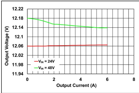
**FIGURE 2-8:** Output Voltage vs. Output Current ( $V_{OUT} = 12V$ ).
