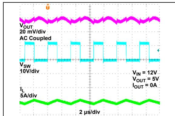
FIGURE 2-47: Switching Waveforms ( $V_{OUT} = 5V$ ,  $I_{OUT} = 0A$ ).
