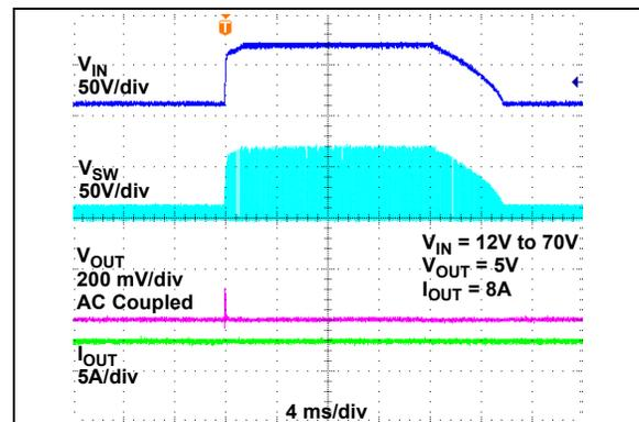
**FIGURE 2-65:** Line Transient Response ( $V_{IN} = 12V$  to  $70V$ ).
