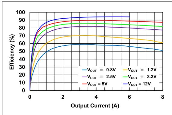
**FIGURE 2-3:** Efficiency vs. Output Current ( $V_{IN} = 48V$ ).
