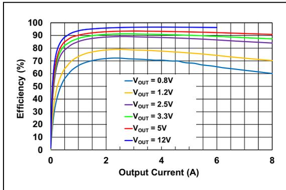
**FIGURE 2-2:** Efficiency vs. Output Current ( $V_{IN} = 24V$ ).
