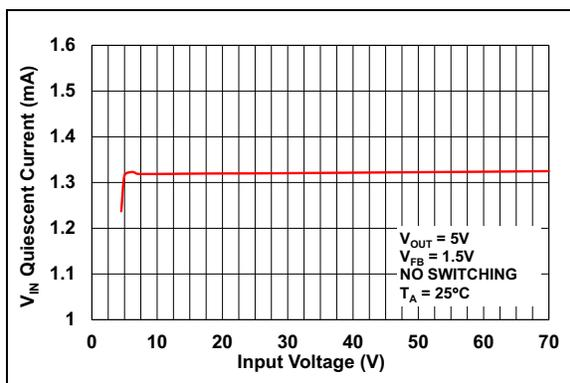
**FIGURE 2-15:**  $V_{IN}$  Quiescent Current vs. Input Voltage.
