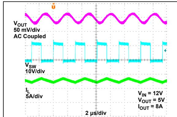
FIGURE 2-48: Switching Waveforms ( $V_{OUT} = 5V$ ,  $I_{OUT} = 8A$ ).
