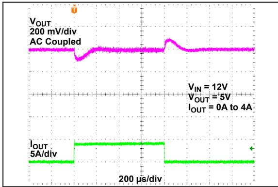
**FIGURE 2-55:** Load Transient Response ( $I_{OUT} = 0A$  to  $4A$ ).
