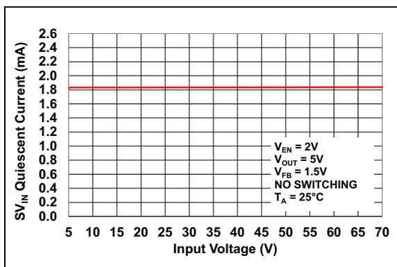
**FIGURE 2-27:**  $SV_{IN}$  Quiescent Current vs. Input Voltage.
