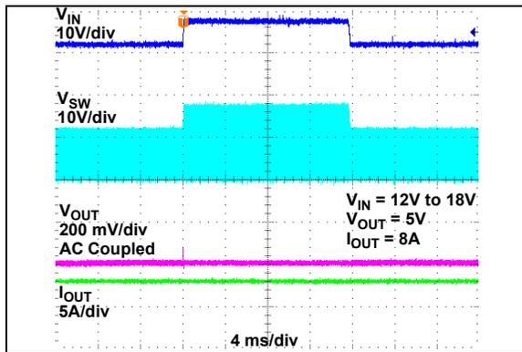
**FIGURE 2-61:** Line Transient Response ( $V_{IN} = 12V$  to  $18V$ ).
