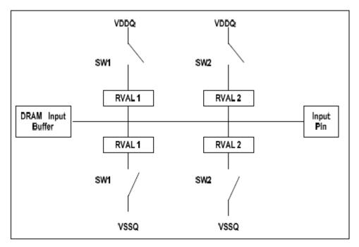
Switch sw1 or sw2 is enabled by the ODT pin. Selection between sw1 or sw2 is determined by "Rtt (nominal)" in EMRS(1) address bits A6 & A2. Target Rtt = 0.5 \* Rval1 or 0.5 \* Rval2.
