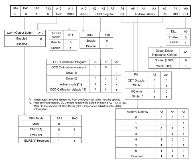
Note1. For DDR2-1066, the "Rtt" must be set to 50 ohm (A2 = 1 & A6 = 1).
