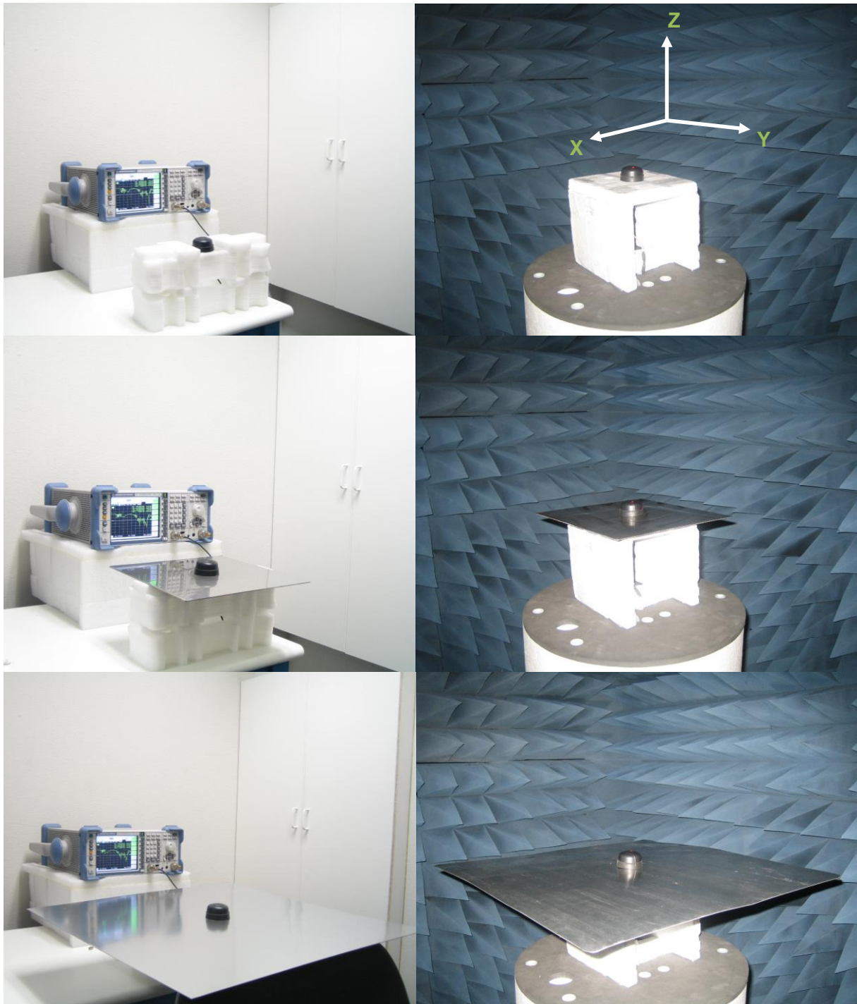
Figure 1. MA106 Antenna test setup in free space, 30x30 cm metal plate and 60x60 cm metal plate, R&S ZVL6 VNA (left) and R&S 4100 CTIA 3D Chamber (Right).
