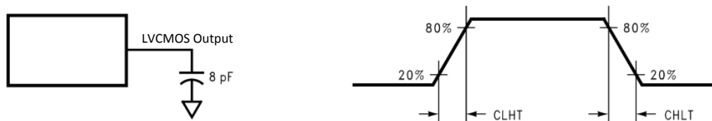
Figure 2. LVC MOS Output Load and Transition Times
