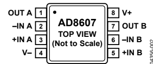
Figure 2. 8-Lead MSOP (RM Suffix)
