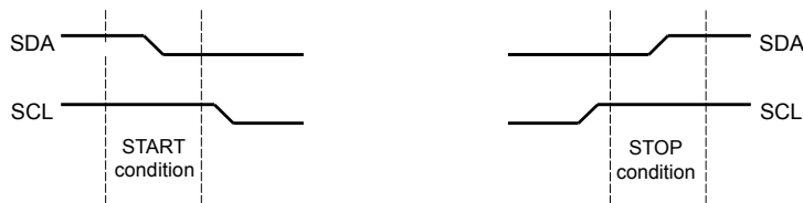
Figure 13-3. START and STOP Conditions
