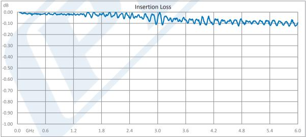
Click the following link (or enter part number in "SEARCH" on website) to obtain additional part information including price, inventory and certifications: 0 dB Fixed Attenuator, QMA Male to QMA Female Brass Tri-Metal Body Rated to 1 Watt Up to 6 GHz PE7AP1002-0
