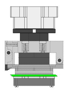
Clamshell lid socket with Torque Indicating Screw Note: Socket Not Included
