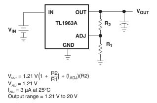
Figure 33. Adjustable Operation
