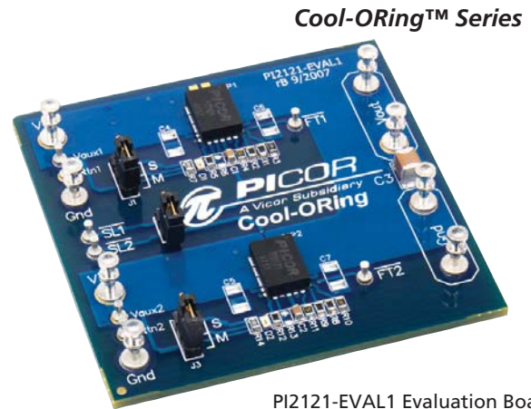
PI2121-EVAL1 Evaluation Board featuring the Cool-ORing PI2121 Full-Function Active ORing Solution.
