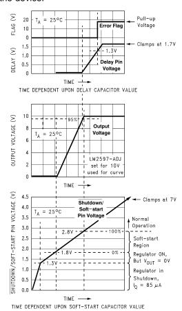
Figure 32. Soft-start, Delay, Error, Output
