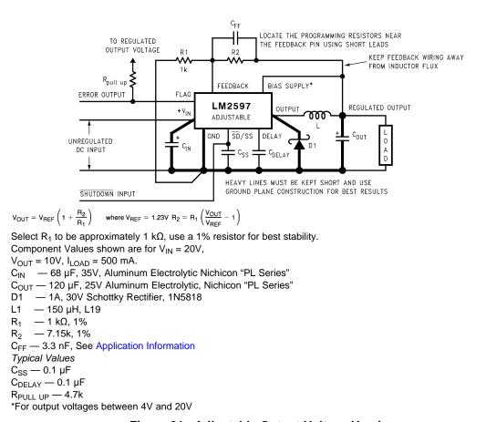
Figure 31. Adjustable Output Voltage Versions
