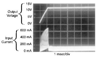
Figure 45. Output Voltage, Input Current, Error Flag Signal, at Start-Up, WITH Soft-start
