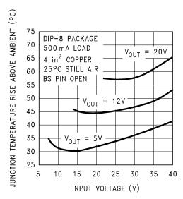
Figure 41. Junction Temperature Rise, PDIP-8
