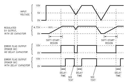
Figure 33. Timing Diagram for 5V Output
