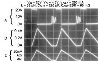
**Discontinuous Mode Switching Waveforms**
