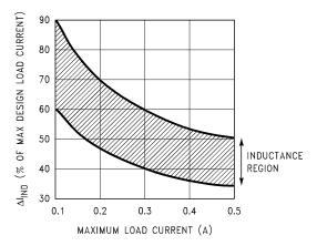
Figure 38. (ΔI<sub>IND</sub>) Peak-to-Peak Inductor Ripple Current (as a Percentage of the Load Current) vs Load Current
