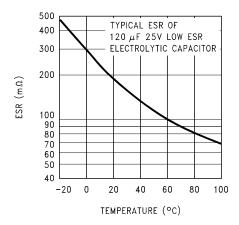
Figure 37. Capacitor ESR Change vs Temperature
