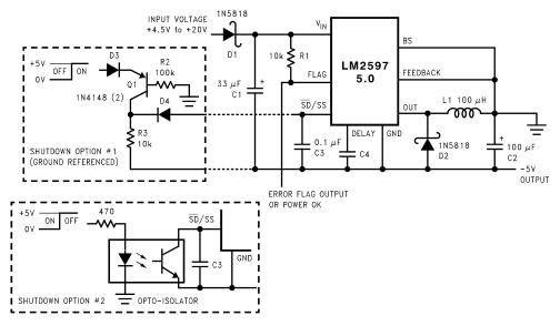
Figure 48. Inverting -5V Regulator With Shutdown and Soft-start
