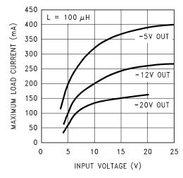
Figure 49. Maximum Load Current for Inverting Regulator Circuit
