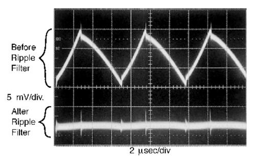
Figure 39. Post Ripple Filter Waveform
