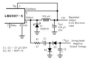
Figure 53. Charge Pump for Generating a Low Current, Negative Output Voltage
