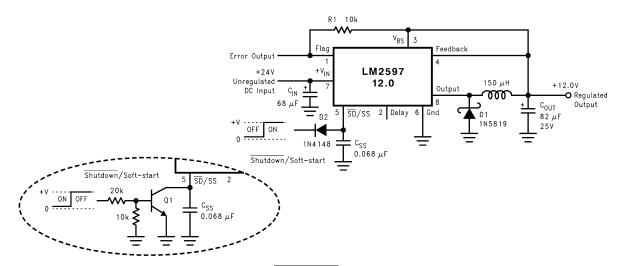
Figure 47. Typical Circuit Using Shutdown /Soft-start and Error Flag Features
