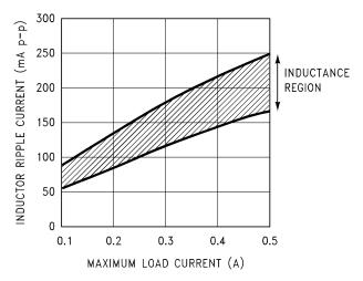
Figure 40. Peak-to-Peak Inductor Ripple Current vs Load Current
