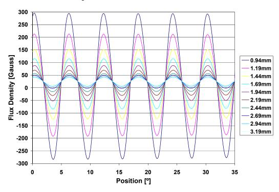
A single curve is distilled from this map data that describes the peak-peak magnetic field versus air gap. Knowing the minimum amount of magnetic flux density that guarantees operation of the sensor, one can determine the maximum operational air gap of the sensor/target system. Referring to the chart below, a minimum required peak-peak signal of 60G corresponds to a maximum air gap of approximately 2.5 mm.
