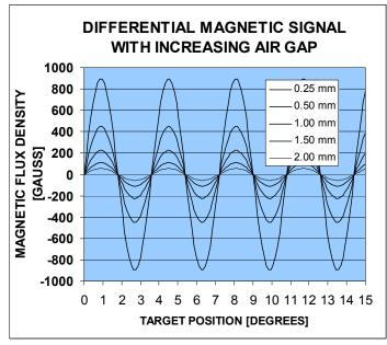
Magnetic Signal with no Amplification
