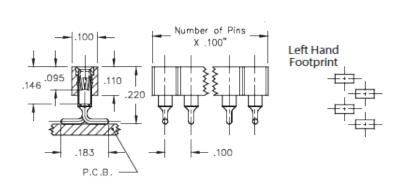
**Description:** Interconnect Socket Surface Mount Socket Accepts .015"- .025" (0,38 - 0,635 mm) dia leads Single Row Surface Mount **Plating Code:** 43 Shell Plating: 200 µ" Tin (matte finish) over 100 µ" Nickel
