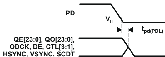
图 8-7. Delay From \overline{PD} Low to Hi-Z Outputs
