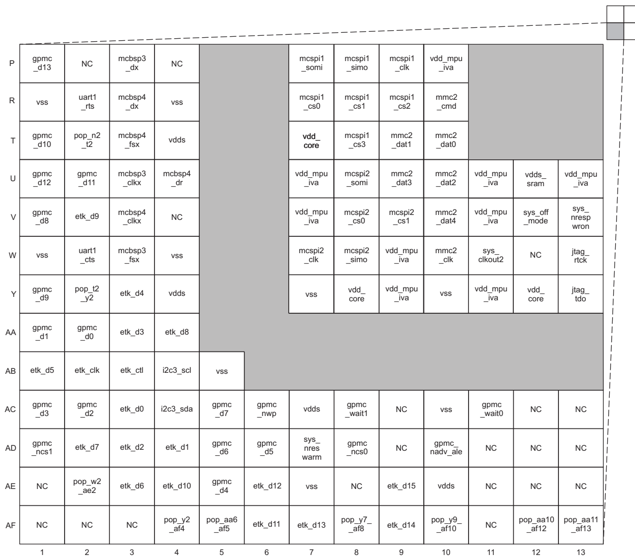
Figure 2-12. CBC Pin Map [Quadrant C - Top View]
