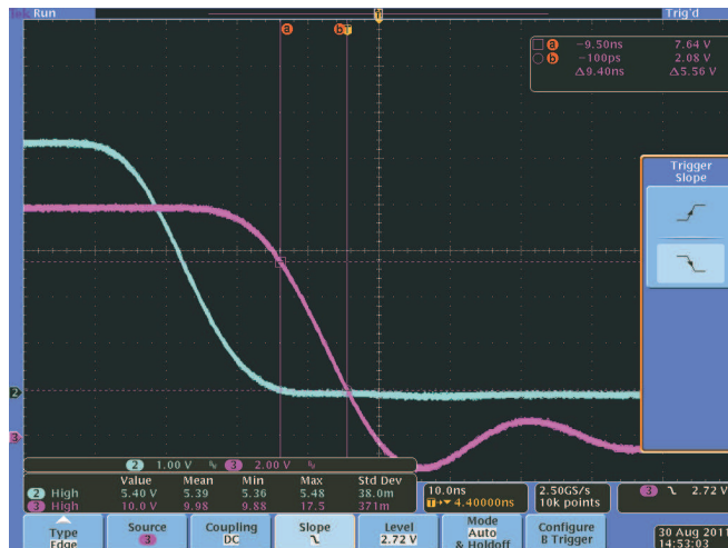
Figure 25. Typical Turn-On Waveform (VDD = 10 V, C_L = 1 nF)
