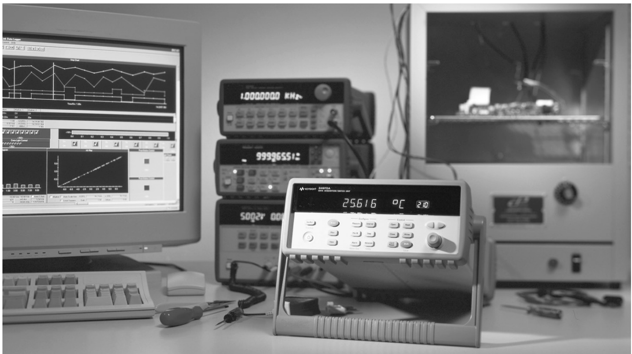
Compact 60-channel data acquisition system
