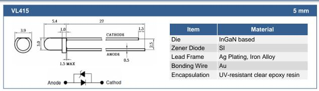
All Dimensions in mm; Tolerance: ±0.15 mm
