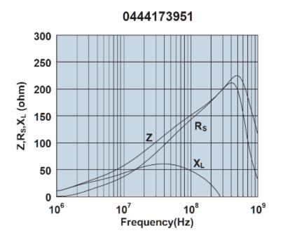
Impedance, reactance, and resistance vs. frequency.
