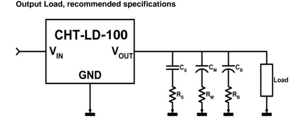
Resistances in series with capacitors represent the internal ESR of these capacitors.
