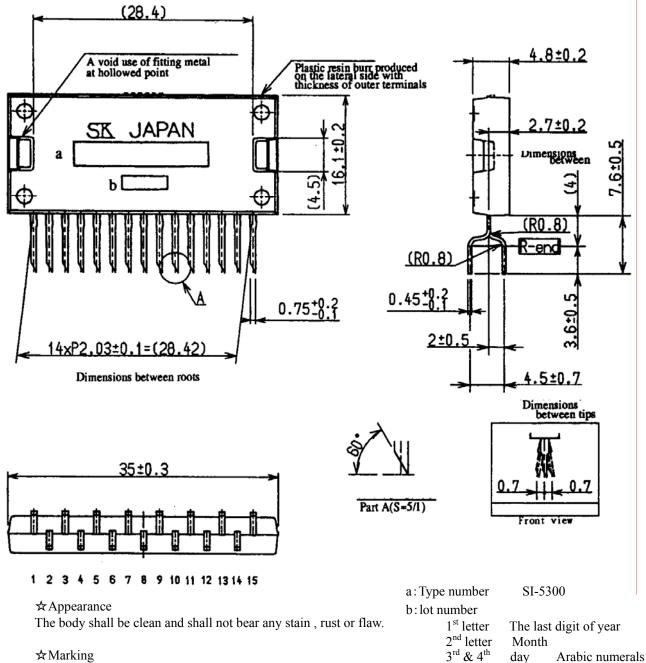
The type number and lot number shall be marked on the body by Laser which shall not be unreadable easily.
