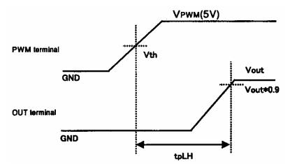
Output transmission time tpLH is time form Vth(2.5Vtyp) of the terminal of PWM to output(Vout\*0.9) of the output terminal.
