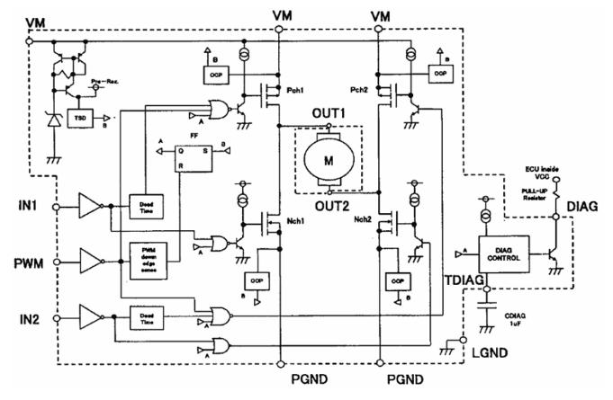
Pre-Reg : Battery inside circuitDead Time : Protection circuit of length currentPWM down edge sence : Detection circuit of PWM signalOCP : Over Current protection circuitTSD : Over temperaturel protection circuitDIAG CONTROL : DIAG control circuit
