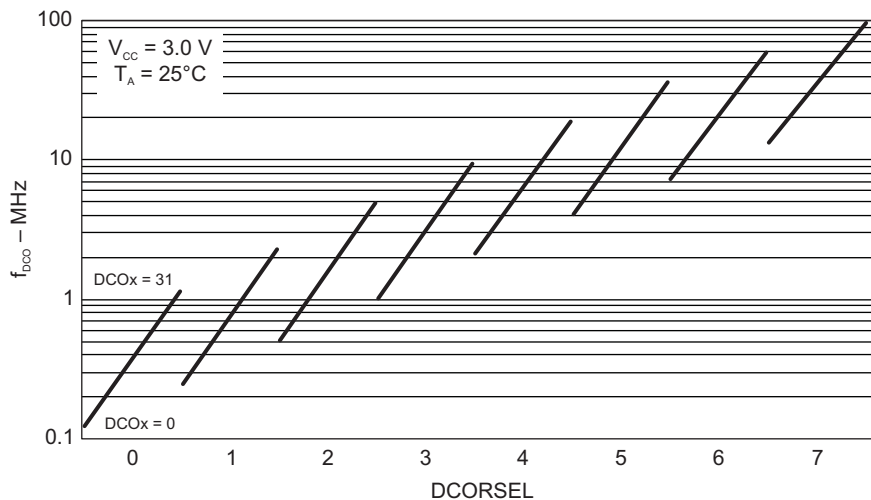
Figure 5-10. Typical DCO Frequency
