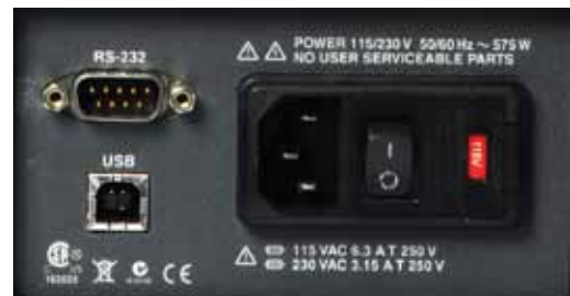
Power and Interface Panel
