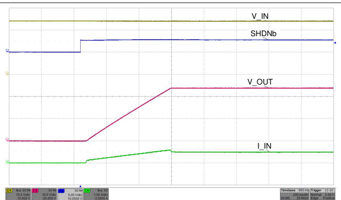
Figure 57. Start-Up With VIN—No Load
