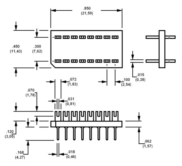
How to order code  $\frac{702\text{-}3728\text{-}01\text{-}\underline{X}\underline{X}\text{-}\underline{00}}{\text{Basic Part No } XX = \text{Plating Finish}}$
