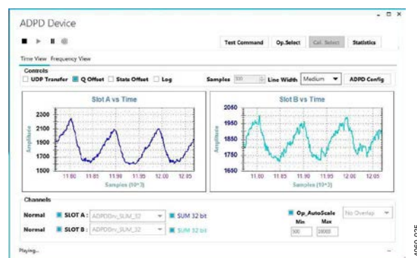
Figure 23. Reflectance PPG Taken Using the Example SpO2 Setup File (see Table 12) Programmed Through Analog Devices Wavetool Software
