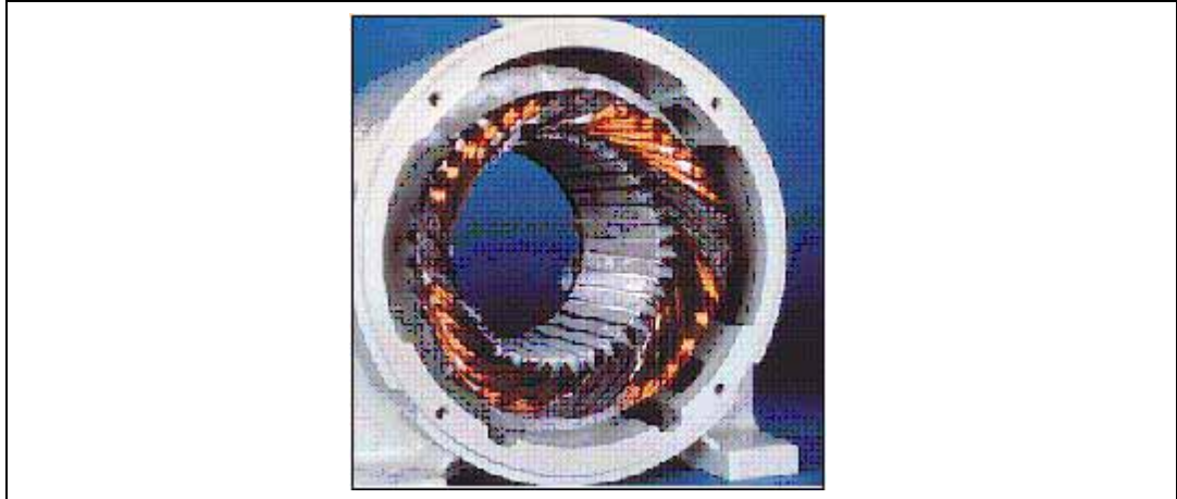
Figure 1. Stator core and windings
