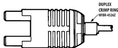
The duplex latching connector is designed for rugged applications requiring greater retention force than the nonlatching duplex connector. When inserting the duplex latching connector into a module, the connector latch mechanism should be aligned with the top surface of the dual combination of horizontal or vertical Versatile Link components. The duplex latching connector is available in gray (HFBR-4516Z).
