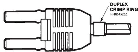
Duplex connectors provide convenient duplex cable termination and are keyed to prevent incorrect insertion into duplex configured modules. The duplex connector is compatible with dual combinations of horizontal or vertical Versatile Link components (e.g., two horizontal transmitters, two vertical receivers, a horizontal transmitter with a horizontal receiver, etc.). The duplex non-latching connector is available in parchment, off-white (HFBR-4506Z).
