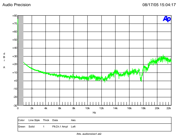
Figure 29 – Audible Noise V_{IN} = 120 VAC; I_{OUT} = 350 mA.
