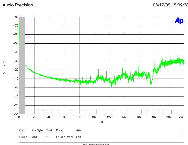
Figure 32 – Audible Noise V_{IN} = 230 VAC; I_{OUT} = 1.2 A.
