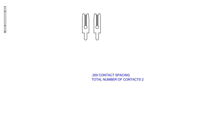
NOTE: CONTACTS ARE HELD IN A CARRIER FOR EASE OF ASSEMBLY
