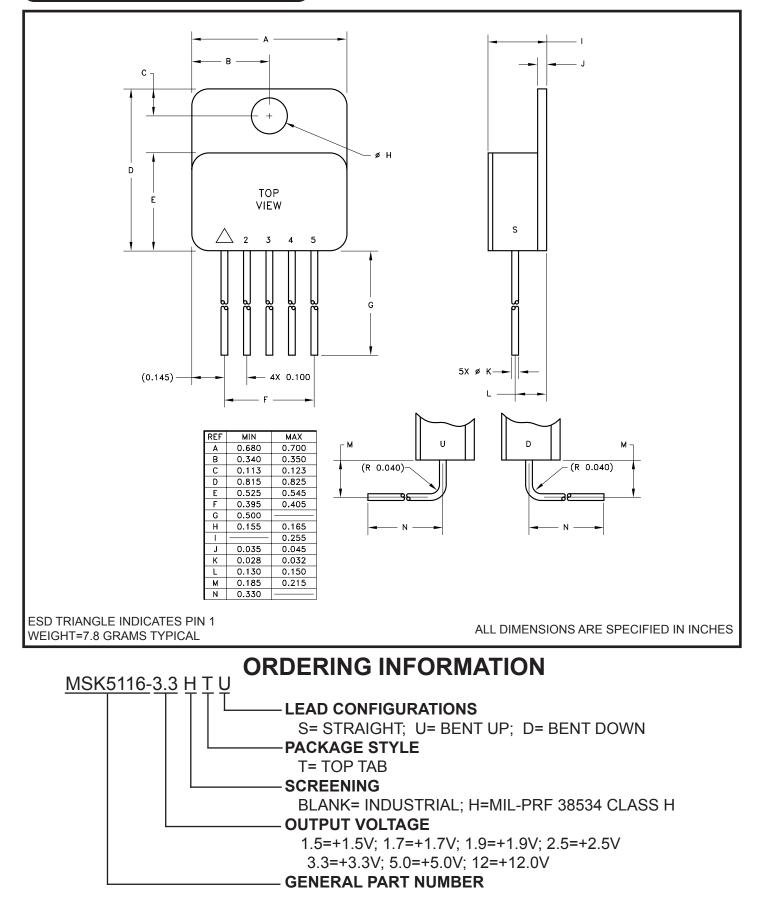
The above example is a +3.3V, Military regulator using the top tab package with leads bent up.
