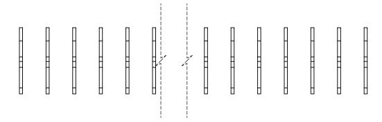
NOTE: CONTACTS ARE HELD IN A CARRIER FOR EASE OF ASSEMBLY
